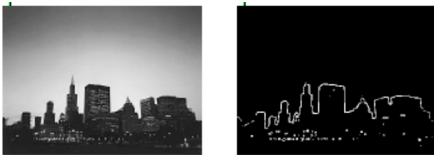
Figure 1. Image before and after applying the Sobel edge detection algorithm.
